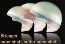
Arai uses a stronger outer shell to spread impact forces and a softer inner shell to absorb remaining energy. The multiple-density EPS inner shell is made using a unique technology of combining three to five densities in various areas as a single component.
